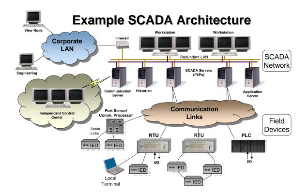
The above diagram depicts a typical Electric Power SCADA system and connections to other networks such as those belonging to backup control centers, the corporate network, and field devices. The focus of this paper and the authentication technology is on the communications links between the SCADA network and field devices.
